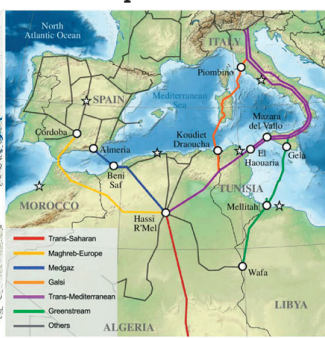
Gas from North-Africa to Europe 60 GW Natural Gas Pipeline capacity 2x0.7 GW Electricity Cable capacity
