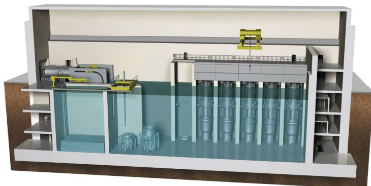
NuScale reactor hall
